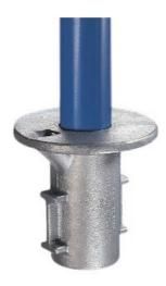
A ground socket fitting for setting in concrete; the posts may either be permanent or removable as required. It incorporates a socket set screw fixing and can be supplied with a plug (sold separately) to fill the hole when the pipe is removed.
