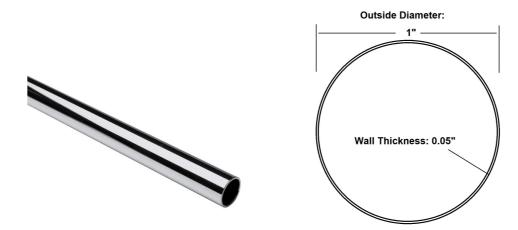
40-A100 architectural round tube is a stainless steel tube with a 1" outside diameter, a 0.05" wall thickness, and is available in stock lengths up to 20 feet. It is made with 304 grade stainless steel.
