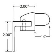
The Bottom Post Horizontal Swivel Bracket is made of cast aluminum and is available in a white painted finish. It is designed to mount on to our 9000/36/F and 9000/42/F receiver posts and will hold the bottom rail of our level picket rail panels 3642L. The bracket swivels from side to side, allowing the panel to be set at an angle other than 180 or 90 degrees.
