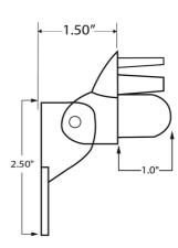
The Top Post Vertical Swivel Bracket is made of cast aluminum and is available in a dark bronze painted finish. It is designed to mount towards the top of our 9000/36/F and 9000/42/F receiver posts and will hold the top rails of our stair picket rail panels 3642S. The bracket swivels up and down, allowing the panels to be set at the standard stair angle of 32.5 degrees.
