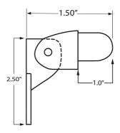
The Bottom Post Vertical Swivel Bracket is made of cast aluminum and is available in a black painted finish. It is designed to mount towards the bottom of our 9000/36/F and 9000/42/F receiver posts and will hold the bottom rails of our stair picket rail panels 3642S. The bracket swivels up and down, allowing the panels to be set at the standard stair angle of 32.5 degrees.
