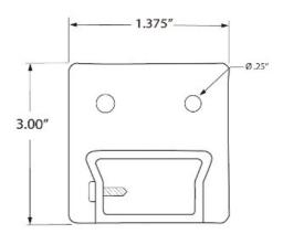
This Bottom Post End Bracket is made of cast aluminum and is in a dark bronze painted finish. It is designed to mount towards the bottom of our 9000/36/F and 9000/42/F receiver posts and will hold the bottom rails of our level picket rail panels 3642L.
