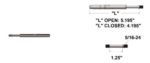
CA-MLT1/8-1 is a tensioning cable fitting for level railing that is designed to mount onto a metal post. It is made of weather resistant 316 grade stainless steel and is designed to hold 1/8" thick cable. This fitting is made in the USA.
