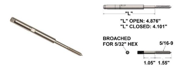
CA-WLT3/16-1 is a tensioning cable fitting for level railing that is designed to mount onto a wood post. It is made of weather resistant 316 grade stainless steel and is designed to hold 3/16" thick cable. This fitting is made in the USA.
