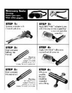
The 00-830/1.3125 splice is an internal tube splice that is made of brass and fits entirely on the inside of a tube. It is designed to connect the ends of two tubes that are 1-5/16"
