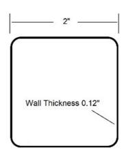
49-C16164 architectural square tube is a stainless steel tube with a 2" width, a 0.12" wall thickness, and is available in stock lengths up to 20 feet. It is made with 316 grade stainless steel.
