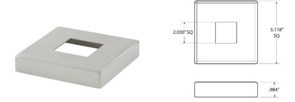
The flange canopy for square tube provides a clean look to your railing post by covering the floor flange and mounting hardware. The canopy is square and has a center hole for 2" square tube and is available in satin (brushed) 316 grade stainless steel.
