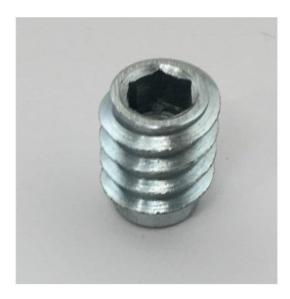
Insert with thread on the outside and the inside. Outside thread goes into wood item# A134. Inside thread allows for bolt of E4586 bracket to fit inside.
