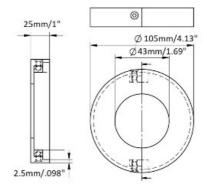
This two-part flange canopy is made of 316 grade stainless steel and has a brushed finish. It is designed to be used with flange item# 49-541/424 and has a design appearance similar to flange canopy item# 49-540/424.
