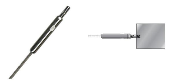
Used on straight runs, this tensioner screws into a drilled and tapped hole in your metal post. Here is a real money-saver, because there is no need for special tees with holes, welded tabs, or any other mounting device. Recommended for level runs using a minimum schedule 80 pipe or square or rectangular steel tubing with a minimum .250" wall.
