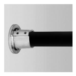
Item 28106 is made of aluminum-magnesium alloy 535 and includes two screws to hold the pipe in place. It is designed to hold 1-1/2" IPS pipe (see item A112ID) and has an anodized finish.
