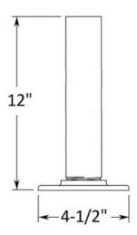
The 20-541/2 flange and insert set is made of cast iron and steel and is designed to mate with 2" round tube (item A120). The flange has four holes for mounting hardware and a large threaded hole in the middle that mates with the threaded end of the insert.
