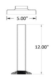
00-B/2 flange, insert, and canopy set is made of a cast iron flange, a steel insert, and a polished brass canopy. This set is designed to mate with 2" OD round tube. The flange has four holes for mounting hardware and a large threaded hole in the middle that mates with the threaded end of the insert.
