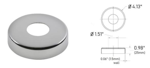
The 47-540/1H round flange canopy or escutcheon plate is made of 316 grade stainless steel, has a polished finish and allows for a 1-1/2" diameter round tube to pass through its center hole. Use this cover as a decorative addition to flanges that are often unseemly because of the mounting hardware used with them.
