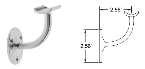
This wall mount handrail bracket is made of 316 stainless steel, has a brushed (satin) finish and is designed to hold 1.67" outside diameter round tube. The back plate has three counter sunk holes that can be positioned for horizontal or angled handrail. Mount this bracket on a wall (recommended on a stud) or on a rectangular vertical post using the included hardware or alternate depending on the material the bracket is being mounted upon.
