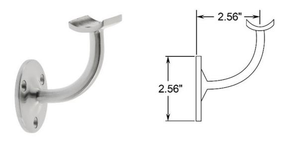
This wall mount handrail bracket is made of 316 stainless steel, has a brushed (satin) finish and is designed to hold 1.67" outside diameter round tube. The back plate has three counter sunk holes that can be positioned for horizontal or angled handrail. Mount this bracket on a wall (recommended on a stud) or on a rectangular vertical post using the included hardware or alternate depending on the material the bracket is being mounted upon.
