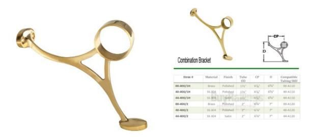
This is our most popular bracket for bar foot rail installation. It is available in three different finishes, for either 1-1/2" or 2" outside diameter tubing. One arm of this bracket mounts to the bar, and the second arm of the bracket rests on the floor to provide additional support.
