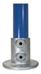
This structural base flange can be used when fixing guard railing or balustrades. There is a single mounting hole located inside the fitting. This allows for a cleaner look. The two set screws in the vertical socket give greater side-load stability to the upright.
