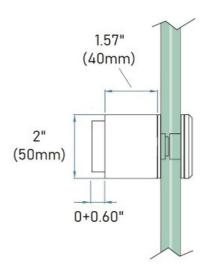
This 2"(50mm) round wall mount glass clamp from IAM Design is made of 304 grade stainless steel, has a brushed (satin) finish and is designed to hold 21/32 – 27/32" thick glass. It has an offset from the wall to the glass of 1.57" (40mm) which can be extended an additional 0.60" (15mm). Mount this bracket on a wall (recommended on a stud) using hardware appropriate for the material that it mounts on.
