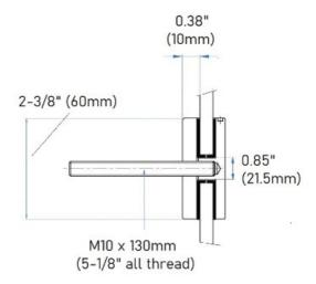
This 2-3/8" round wall mount glass clamp from IAM Desgin is made of 316 grade stainless steel, has a brushed (satin) finish and is designed to hold 5/16 - 21/32" thick glass. It has an offset from the wall to the glass of 0.38" (10mm) and comes complete with a threaded bolt. Mount this bracket on a wall (recommended on a stud) or on a rectangular vertical post using the included hardware or alternate depending on the material the bracket is being mounted upon.
