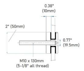
This 2"round wall mount glass clamp from IAM Design is made of 316 grade stainless steel, has a brushed (satin) finish and is designed to hold 5/16 - 21/32" thick glass. It has an offset from the wall to the glass of 0.38" (10mm) and comes complete with a threaded bolt. Mount this bracket on a wall (recommended on a stud) or on a rectangular vertical post using the included hardware or alternate depending on the material the bracket is being mounted upon.
