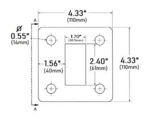
This floor mount flange is made of 316 grade stainless steel, has a mill finish and is designed to hold 2.36" x 0.78" rectangular tube. Weld the tube to the flange (do not use adhesive or fasteners). It has four thru holes to mount on the floor using appropriate hardware for the material that the flange is being mounted upon.
