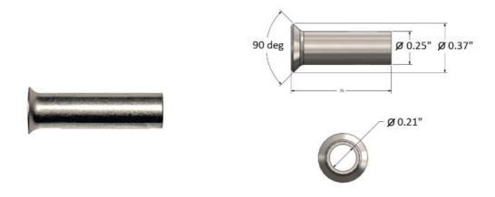
To keep the cable from biting in the wood, the stainless steel post protector tube is inserted into a wood post where the cable enters/exits the post at an angle. See drawings for details.
