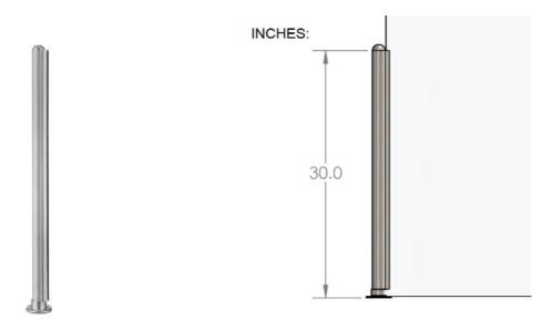
The 44-PR55/E Divider Booth Post is made of brushed (satin) 304 grade stainless steel, 1-1/2" round tube, has a height of 30", and is designed to hold a ¼" thick panel. Each post comes with a half-ball end cap on top, a round flange attached at the bottom, and one u-channel that holds a panel in place.
