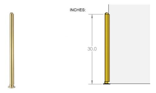
The 00-PR55/E Divider Booth Post is made of brass, 1-1/2" round tube, has a height of 30", and is designed to hold a ¼" thick panel. Each post comes with a half-ball end cap on top, a round flange attached at the bottom, and one u-channel that holds a panel in place.
