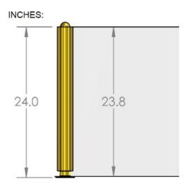
The 00-PR53/C Divider Booth Post is made of polished brass, 1-1/2" round tube, has a height of 24", and is designed to hold ¼" thick panels. Each post comes with a half-ball end cap on top, a round flange attached at the bottom, and a two u-channels to hold panels in place.
