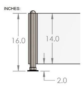
The 44-PR51/C Divider Booth Post is made of brushed (satin) 304 grade stainless steel, 1-1/2" round tube, has a height of 16", and is designed to hold ¼" thick panels. Each post comes with a half-ball end cap on top, a round flange attached at the bottom, and two u-channels that hold the panels in place.
