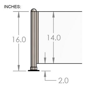
The 44-PR51/E Divider Booth Post is made of brushed (satin) 304 grade stainless steel, 1-1/2" round tube, has a height of 16", and is designed to hold a ¼" thick panel. Each post comes with a half-ball end cap on top, a round flange attached at the bottom, and onechannel that holds a panel in place.
