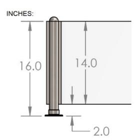
The 40-PR53/C Divider Booth Post is made of polished 304 grade stainless steel, 1-1/2" round tube, has a height of 20", and is designed to hold %" thick panels. Each post comes with a half-ball end cap on top, a round flange attached at the bottom, and two u-channels that hold the panels in place.
