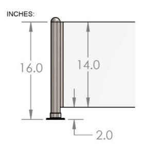
The 40-PR51/E Divider Booth Post is made of polished 304 grade stainless steel, 1-1/2" round tube, has a height of 16", and is designed to hold a ¼" thick panel. Each post comes with a half-ball end cap on top, a round flange attached at the bottom, and one u-channel that holds a panel in place.
