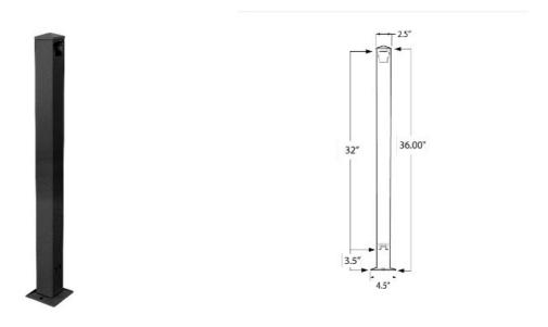
This 36" High Floor Mount End Post is a 2-1/2" square aluminum post that has two machined holes that are designed to receive the top and bottom rails of one picket rail panel. This post has a black paint finish.
