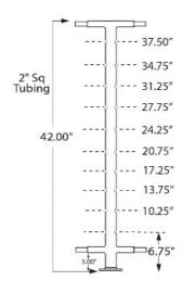
These CS508 prefabricated posts are 2" square posts, 42" high for cable rail and are made of aluminum. They include pre-drilled holes, a welded flange, and necks on the top and the bottom to fit with rectangular tube 2" x 1". Cable kits are available in both 1/8" and 3/16" thickness.
