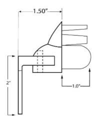
The Top Post Horizontal Swivel Bracket is made of cast aluminum and is available in a dark bronze painted finish. It is designed to mount on to our 9000/36/F and 9000/42/F receiver posts and will hold the top top rail of our level picket rail panels 3642L. The bracket swivels from side to side, allowing the panels to be set at an angle other than 180 or 90 degrees.
