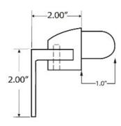
The Bottom Post Horizontal Swivel Bracket is made of cast aluminum and is available in a black painted finish. It is designed to mount on to our 9000/36/F and 9000/42/F receiver posts and will hold the bottom rail of our level picket rail panels 3642L. The bracket swivels from side to side, allowing the panel to be set at an angle other than 180 or 90 degrees.
