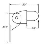
The Bottom Post Vertical Swivel Bracket is made of cast aluminum and is available in a dark bronze painted finish. It is designed to mount towards the bottom of our 9000/36/F and 9000/42/F receiver posts and will hold the bottom rails of our stair picket rail panels 3642S. The bracket swivels up and down, allowing the panels to be set at the standard stair angle of 32.5 degrees.
