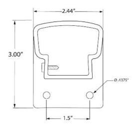
This Top Post End Bracket is made of cast aluminum and is in a dark bronze painted finish. It is designed to mount towards the top of our 9000/36/F and 9000/42/F receiver posts and will hold the top rails of our level picket rail panels 3642L.
