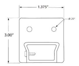
This Bottom Post End Bracket is made of cast aluminum and is in a black painted finish. It is designed to mount towards the bottom of our 9000/36/F and 9000/42/F receiver posts and will hold the bottom rails of our level picket rail panels 3642L.
