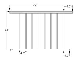
This 6ft long Level Picket Rail Panel is designed for 36" high railing and it has 3/4" square pickets that are spaced 3-3/4" apart to pacify the 4" sphere rule. This panel has a white painted finish.
