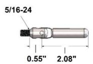
CA-MSN3/16-1 is a non-tensioning cable fitting for level railing that is designed to mount onto a metal post. This fitting has a swivel feature that allows the cable to be set at an angle. It is made of weather resistant 316 grade stainless steel and is designed to hold 3/16" thick cable. This fitting is made in the USA.
