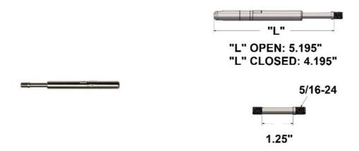
CA-MLT3/16-1 is a tensioning cable fitting for level railing that is designed to mount onto a metal post. It is made of weather resistant 316 grade stainless steel and is designed to hold 3/16" thick cable. This fitting is made in the USA.
