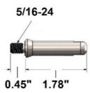
CA-MLN3/16-1 is a non-tensioning cable fitting for level railing that is designed to mount onto a metal post. It is made of weather resistant 316 grade stainless steel and is designed to hold 3/16" thick cable. This fitting is made in the USA.
