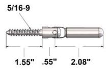
CA-WSN3/16-1 is a non-tensioning cable fitting for stair railing that is designed to mount onto a wood post. This fitting has a swivel feature that allows the cable to be set at an angle. It is made of weather resistant 316 grade stainless steel and is designed to hold 3/16" thick cable. This fitting is made in the USA.
