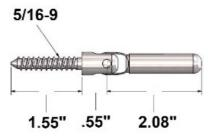
CA-WSN1/8-1 is a non-tensioning cable fitting for stair railing that is designed to mount onto a wood post. This fitting has a swivel feature that allows the cable to be set at an angle. It is made of weather resistant 316 grade stainless steel and is designed to hold 1/8" thick cable. This fitting is made in the USA.
