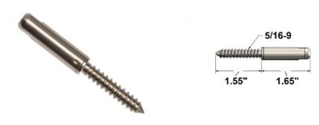
CA-WLN1/8-1 is a non-tensioning cable fitting for level railing that is designed to mount onto a wood post. It is made of weather resistant 316 grade stainless steel and is designed to hold 1/8" thick cable. This fitting is made in the USA.
