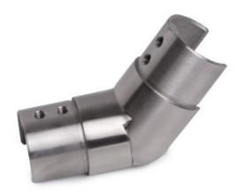
This adjustable elbow for channel tube is made of 316 grade stainless steel and has a brushed finish. It is designed to connect two different ends of 1.67" diameter channel tube, item# A114U and enables an upward bend in the tube. Connect the elbow to the tube ends using our adhesive and activator (items LB-00201 and 00211).
