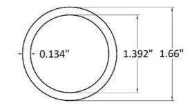
1.66" x 10 gauge Mechanical Tube has the following sizing
