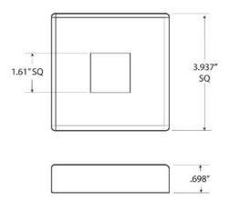
The flange canopy for square tube provides a clean look to your railing post by covering the floor flange and mounting hardware. The canopy is square and has a center hole for 1.57" square tube and is available in satin (brushed) 316 grade stainless steel.
